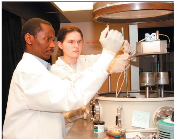
Dr. Tom Oder and student Pam Martin work at the YSU Sputter Deposition System, which under high heat will improve the physical and electrical qualities of metal films deposited on semiconductors.
